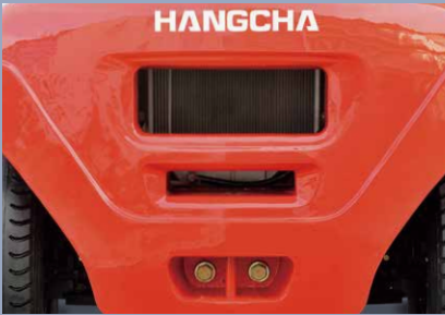
Enlarged heat dissipation channels and double-channel vents are used to ensure normal water and oil temperature. An independent hydraulic oil heat dissipater is provided, which meets the requirements of harsh operating conditions
