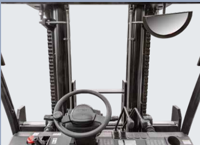
The enhanced mast, frame and steering axle improve the impact resistance of the vehicle
